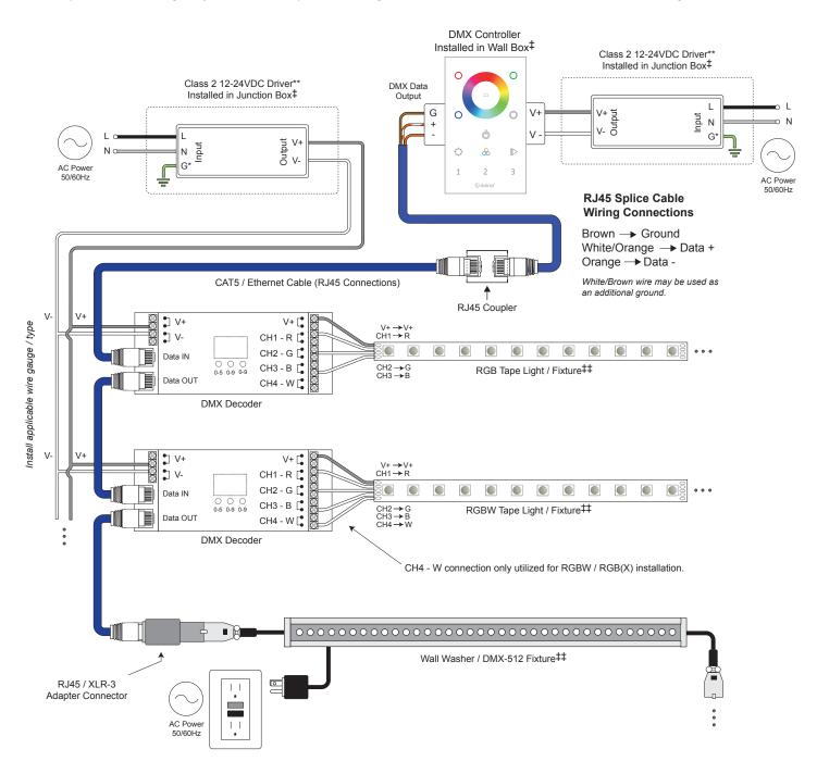
\* Driver may not require a fault ground connection. Refer to driver specifications for additional information.
